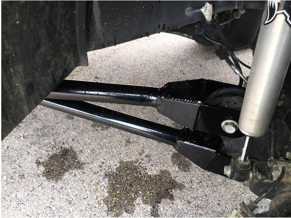
Now install the lower arm, starting with the axle end first and then raising the adjustable Johnny Joint side into the factory radius arm bracket on the frame, using the factory hardware on both ends. Again, you may need to adjust the joint to get the bolt holes to line up.
