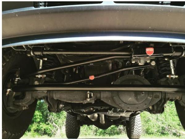
Steering installed in a stock 3" configuration, with the drag link above the stock pitman arm.
