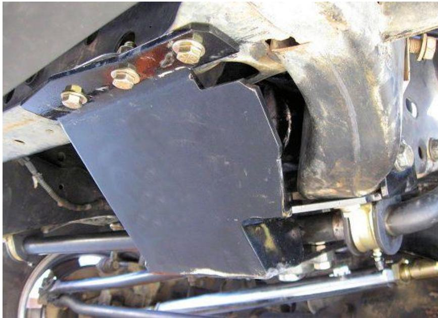
Thank you for purchasing the Dodge Off Road Steering Brace, the strongest and best-designed steering brace on the market for Dodge Ram trucks! This brace is used to support your steering box from the push and pull design of Dodge steering, while eliminating the transfer of frame flex to the sector shaft, which is a problem that all frame-to-frame braces cause.
