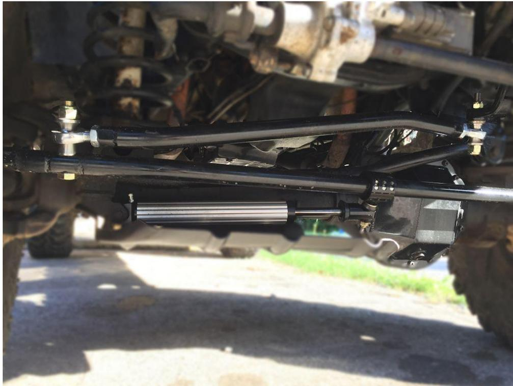
Steering installed in a 3" to 6" configuration, with the drag link below the pitman arm. This is done using a drop pitman arm that has a reverse taper, required on all lift heights over 4".
